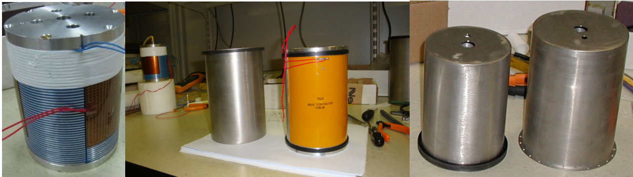
Fig. 4. From left to right: C-field coils (in blue) and inner heater; first magnetic shield and external heater; the outmost magnetic shields.
